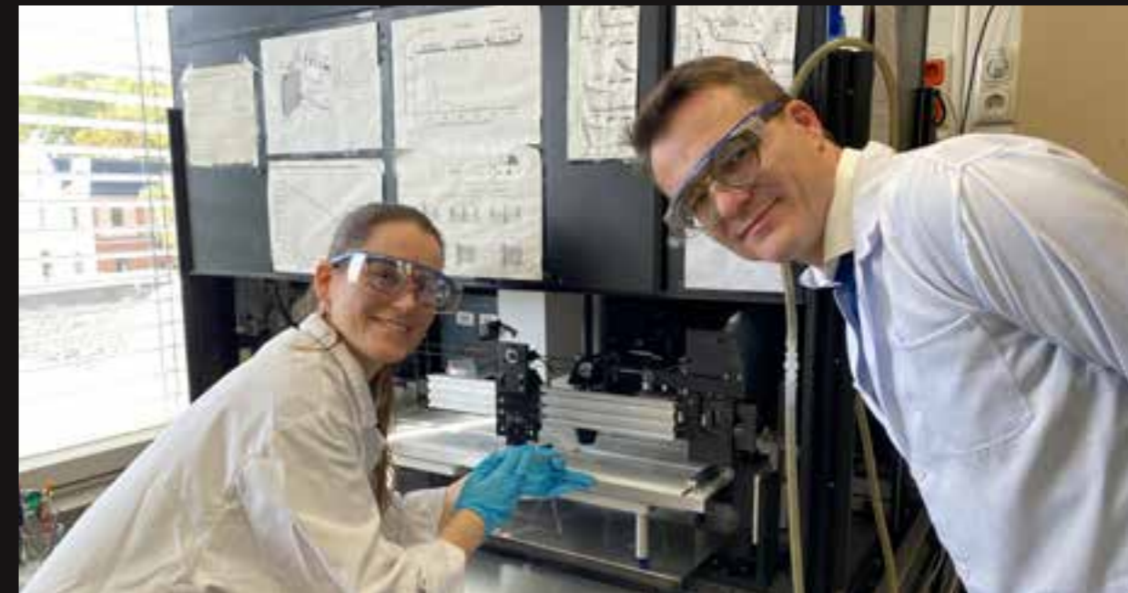
Dr. Sarah Jasmin Finkelmeyer and PD Dr. habil Martin Presselt at the setup, which can be used to produce thin films with specific properties that are used, for example, in the production of improved flexible solar cells. © Katrin Uhlig
