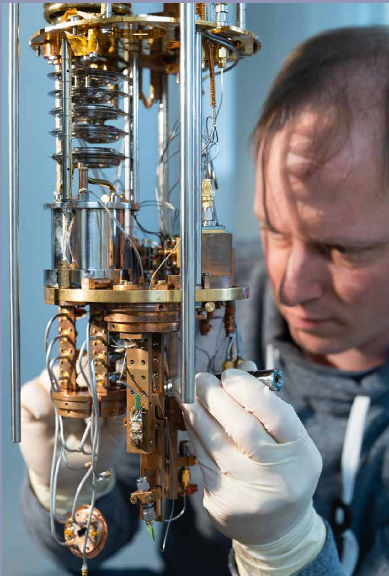
Dr. Gregor Oelsner, head of the Quantum Circuits Group in the Quantum Systems Research Department and subproject leader of QSolid at Leibniz IPHT, prepares the cryostat for ultra-low temperatures for the research on new superconducting circuits for the quantum computer of the future.
