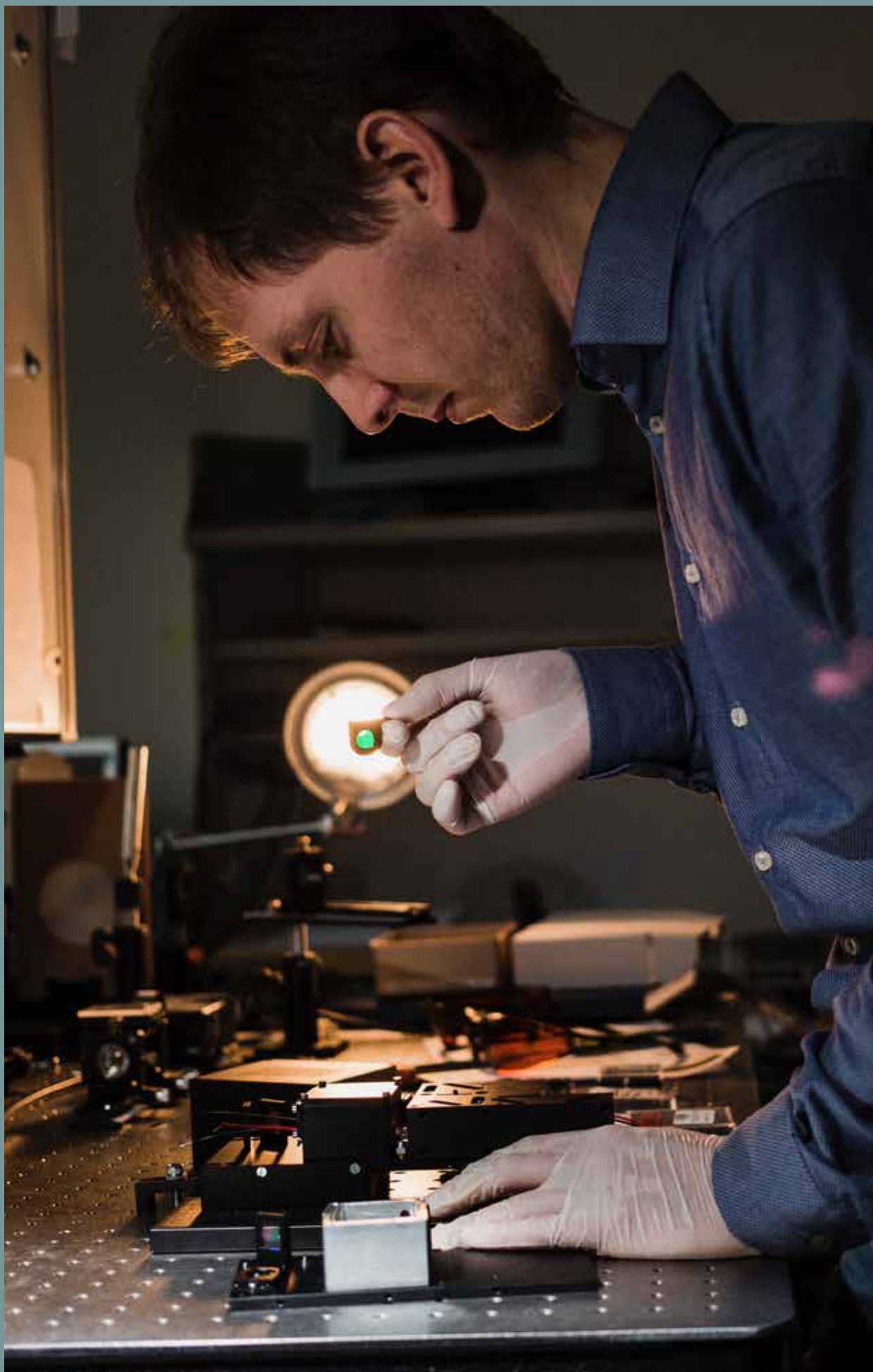
Henry John, engineer in the Sensor Research and Systems Integration Group at Leibniz IPHT, places the optical gratings in the Raman2Go system with great sensitivity.
