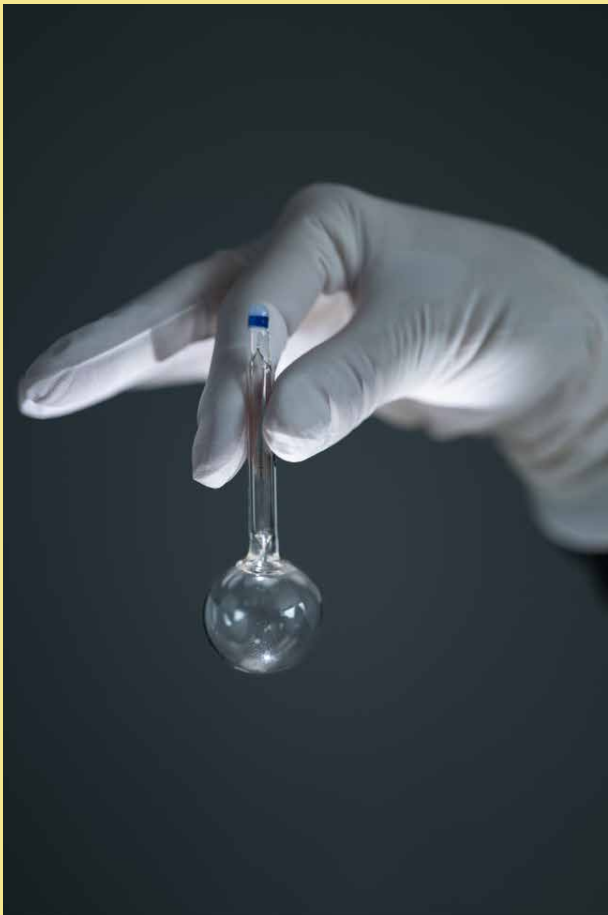
The atoms are located in a special glass vapor cell that tracks signals from the exotic matter in a magnetically very well-shielded setup.
