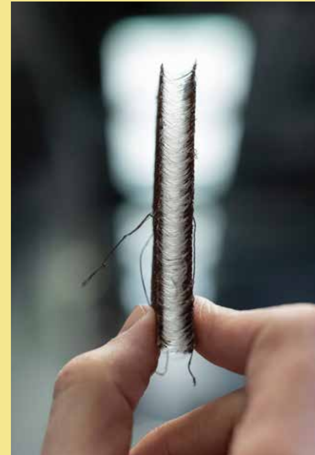
Clever fabric: 3D spacer fabrics made of polyester, thermoelectrically coated as well as equipped with copper contacts, are the starting point for smart clothing suitable for energy generation and active cooling. © Sven Döring
