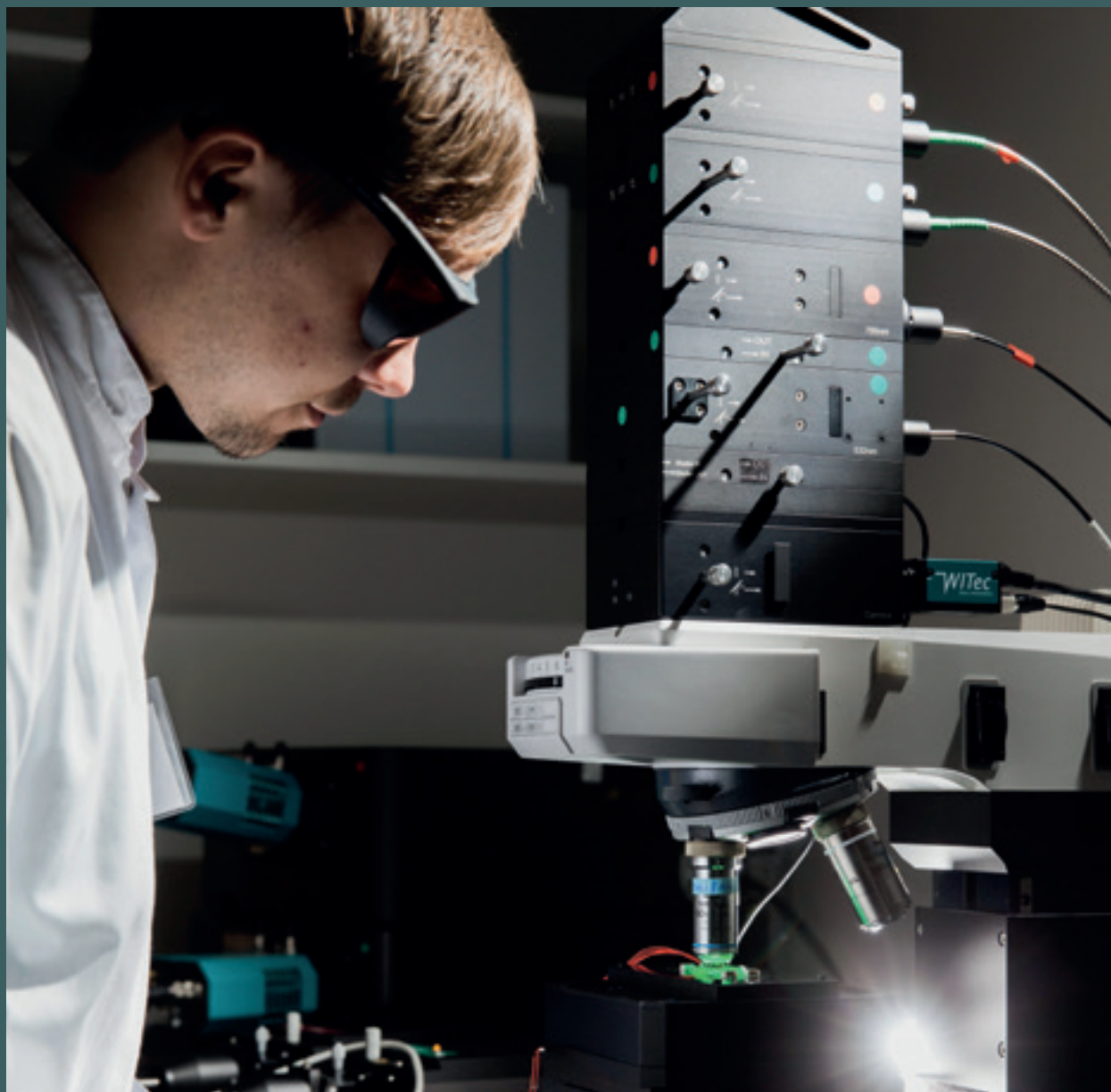
Using a Raman microspectroscope, PhD student Marcel Dahms records the specific vibrational spectra of bacteria trapped on a chip.
