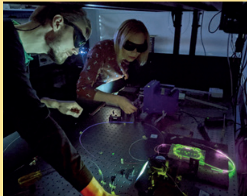
Maria Chernysheva and PhD student Dennis Kirsch during an experiment with a Tm fiber laser (purple), which is pumped by an erbium fiber laser (green) is pumped. © Leibniz IPHT
