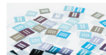
Depending on the thickness of the aluminum oxide layer, the chips shimmer in different colors. © Sven Döring
